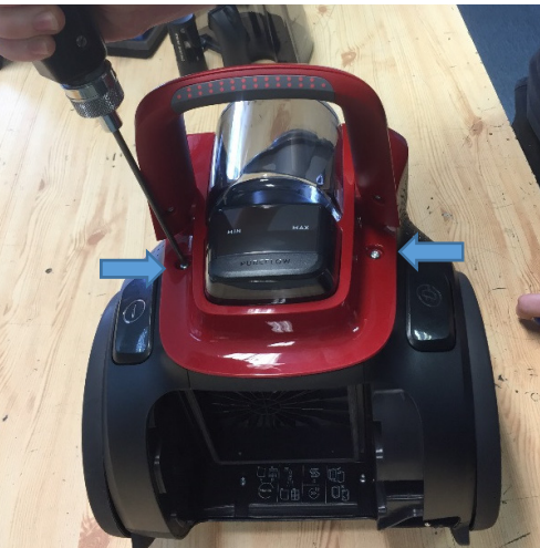
06. Remove the screws.
