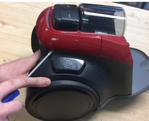
07. Snap out the handle around the cyclone using the screwdriver.
