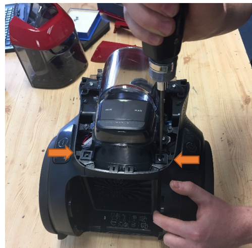
08. Remove the screws.
