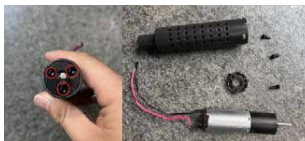
10. Remove the screws and take out the front cover of the motor.
