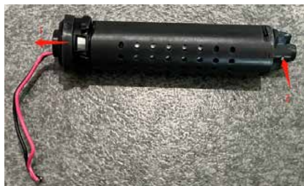
09. First, remove the bearing bracket in the direction of the arrow at point 1, and then push the shaft in the direction of the arrow at point 2 to remove the roller brush drive bracket.
