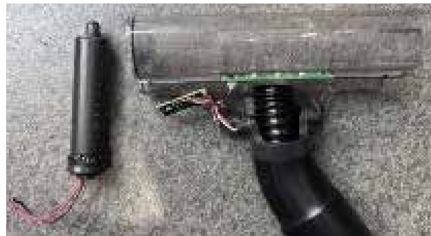
09. First, remove the bearing bracket in the direction of the arrow at point 1, and then push the shaft in the direction of the arrow at point 2 to remove the roller brush drive bracket.
