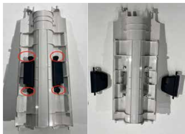
08. Follow the arrow direction to remove the PCB Aholder.
