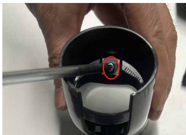
27. Press the button and take out the joint bracket
