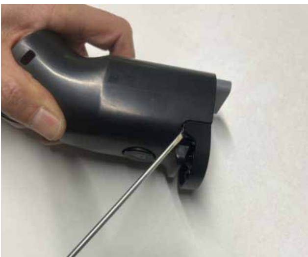
25. Press the hook and take out the pedal.
