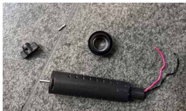
10. Remove the screws and take out the front cover of the motor.
