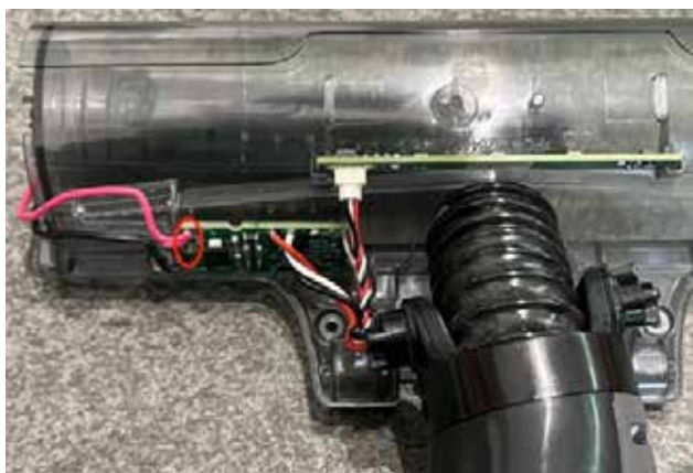
08. Cut the motor wires connected to the PCB.
